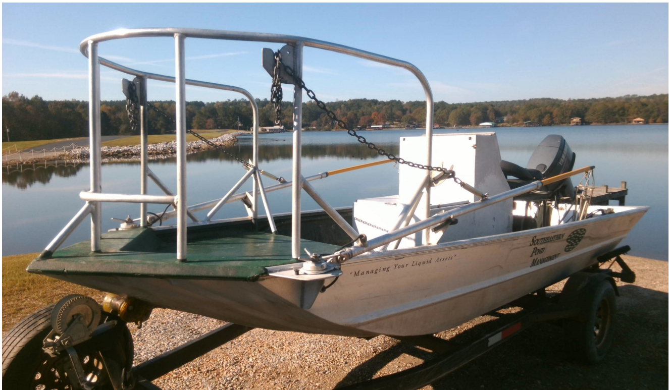
Electrofishing equipment was used to collect a fish sample from Lake Eddins, November 2019.
